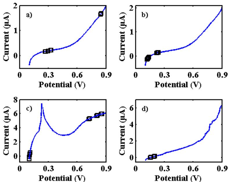
Figure 11. Variables selected to a) Cysteine determination using AuAT electrode. b) Glutathione determination using AuAT. c) Glutathione determination using CNT electrode. d) Glutathione determination using AuBT electrode.
