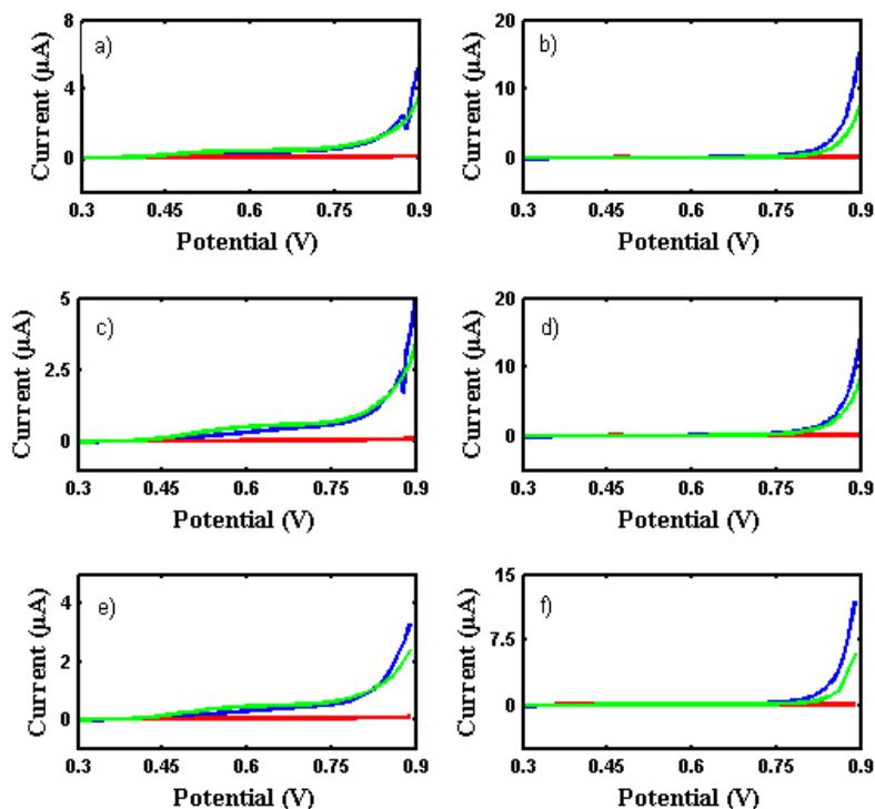
Figure 3. Voltammograms obtained. (AuAT — / CAR — / AuBT —). a) Cysteine with potential step of 0.001V. b) Glutathione with potential step of 0.001V. c) Cysteine with potential step of 0.002V. d) Glutathione with potential step of 0.002V. e) Cysteine with potential step of 0.01V. f) Glutathione with potential step of 0.01V
