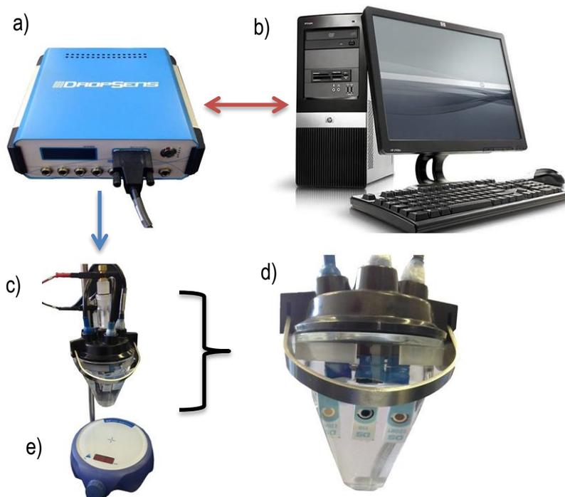
Figure 2. Instrumentation for the experiment. a) Multi Potentiostat / Galvanostat DropSens. b) PC equipped with Drop View software. c) Electrolytic cell. d) Electrolytic cell in perspective, showing the screen-printed electrodes. e) Magnetic stirrer.
