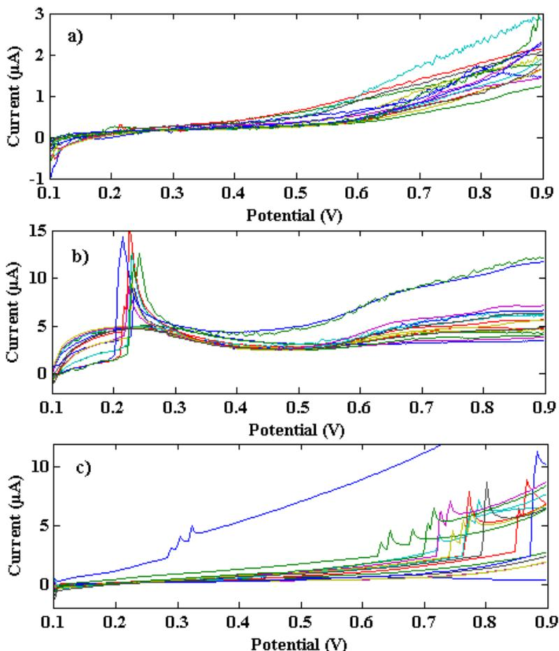
Figure 10. Voltammograms obtained by a) AuAT b) CNT c) AuBT
