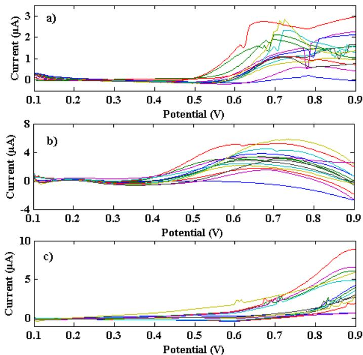
Figure 12. Voltammograms obtained by a) AuAT. b) CNT. c) AuBT.
